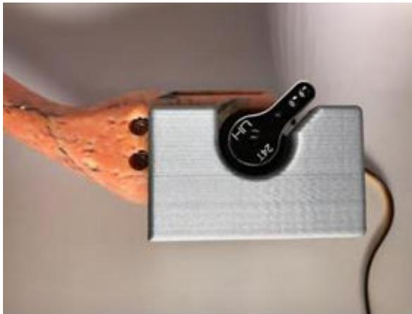
Figure 6: The 3D printed mechanical jig (grey) is placed on the motor and guides the coupling of the servo horn (black) to the proper orientation.
