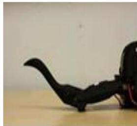
The femur is lowered until it touches the flat surface at its lowest point. The PWM period of this point is recorded
